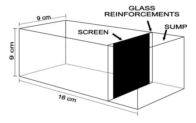
Figure 1. Glass chamber with sump area. Modified from Norberg and Mount (1985). From USEPA (1987c).
