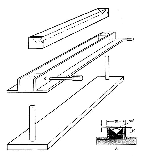
(A) Cross-section of 250 mm long mould
