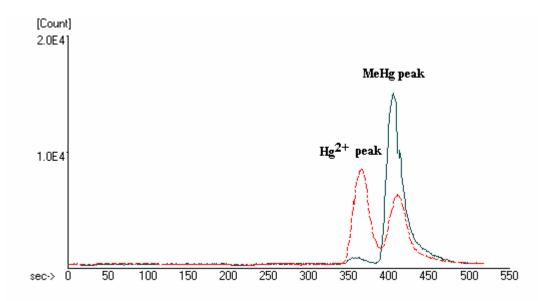
Solid line: A methyl mercury standard in acid solution before the addition of iron Dash line: A methyl mercury standard in acid solution with 500 ppm iron.
