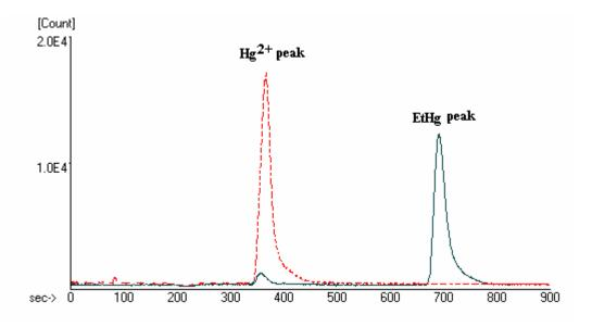
Solid line: An ethyl mercury standard in acid solution without the addition of iron Dash line: An ethyl mercury standard in acid solution with 500 ppm iron.
