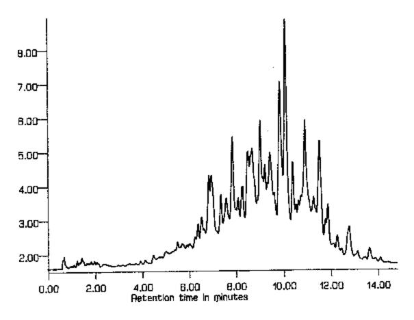
Toxaphene analyzed on an SPB-608 fused-silica open-tubular column. The GC operating conditions were as follows: 30-m x 0.53-mm ID SPB-608. Temperature program: 200EC (2 min hold) to 290EC at 6EC/min.
