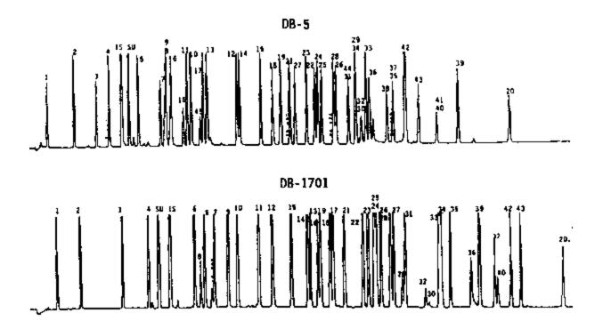
Organochlorine pesticides analyzed on a DB-5/DB-1701 fused-silica open-tubular column pair. The GC operating conditions were as follows:  $30\text{-m} \times 0.53\text{-mm}$  ID DB-5 ( $0.83\text{-}\mu\text{m}$  film thickness) and  $30\text{-m} \times 0.53\text{-mm}$  ID DB-1701 ( $1.0\text{-}\mu\text{m}$  film thickness) connected to an 8-in. injection tee (Supelco Inc.). Temperature program: 140EC (2min hold) to 270EC (1min hold) at 2.8EC/min.
