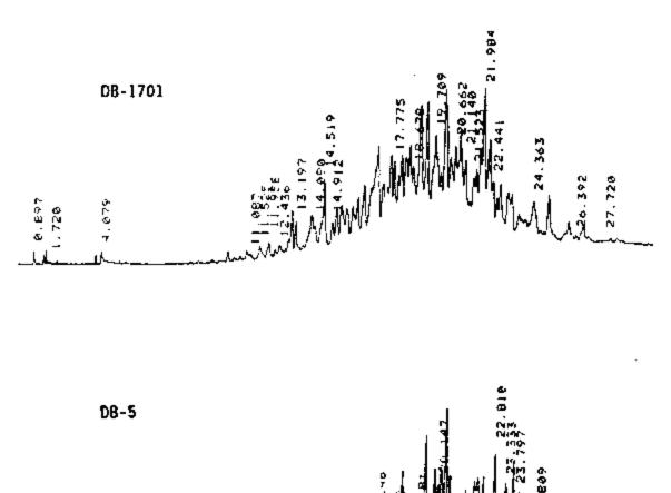
Strobane analyzed on a DB-5/DB-1701 fused-silica open-tubular column pair. The GC operating conditions were as follows:  $30-m \times 0.53-mm$  ID DB-5 (1.5- $\mu$ m film thickness) and  $30-m \times 0.53-mm$  ID DB-1701 (1.0- $\mu$ m film thickness) connected to a J&W Scientific press-fit Y-shaped inlet splitter. Temperature program: 150EC (0.5 min hold) to 190EC (2 min hold) at 12EC/min then to 275EC (10 min hold) at 4EC/min.
