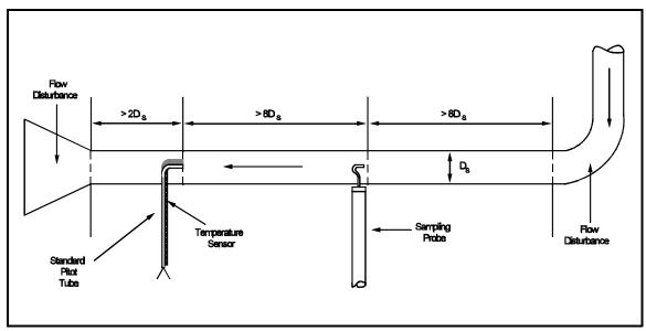
Figure 1A-1. Recommended sampling arrangement for small ducts
