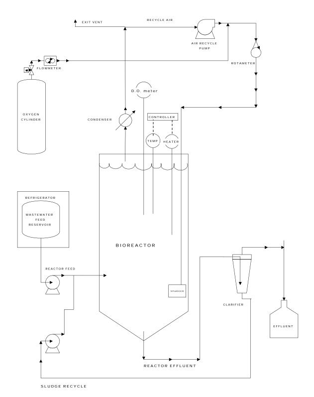
EPA METHOD 304A VENT BIOREACTOR SYSTEM
